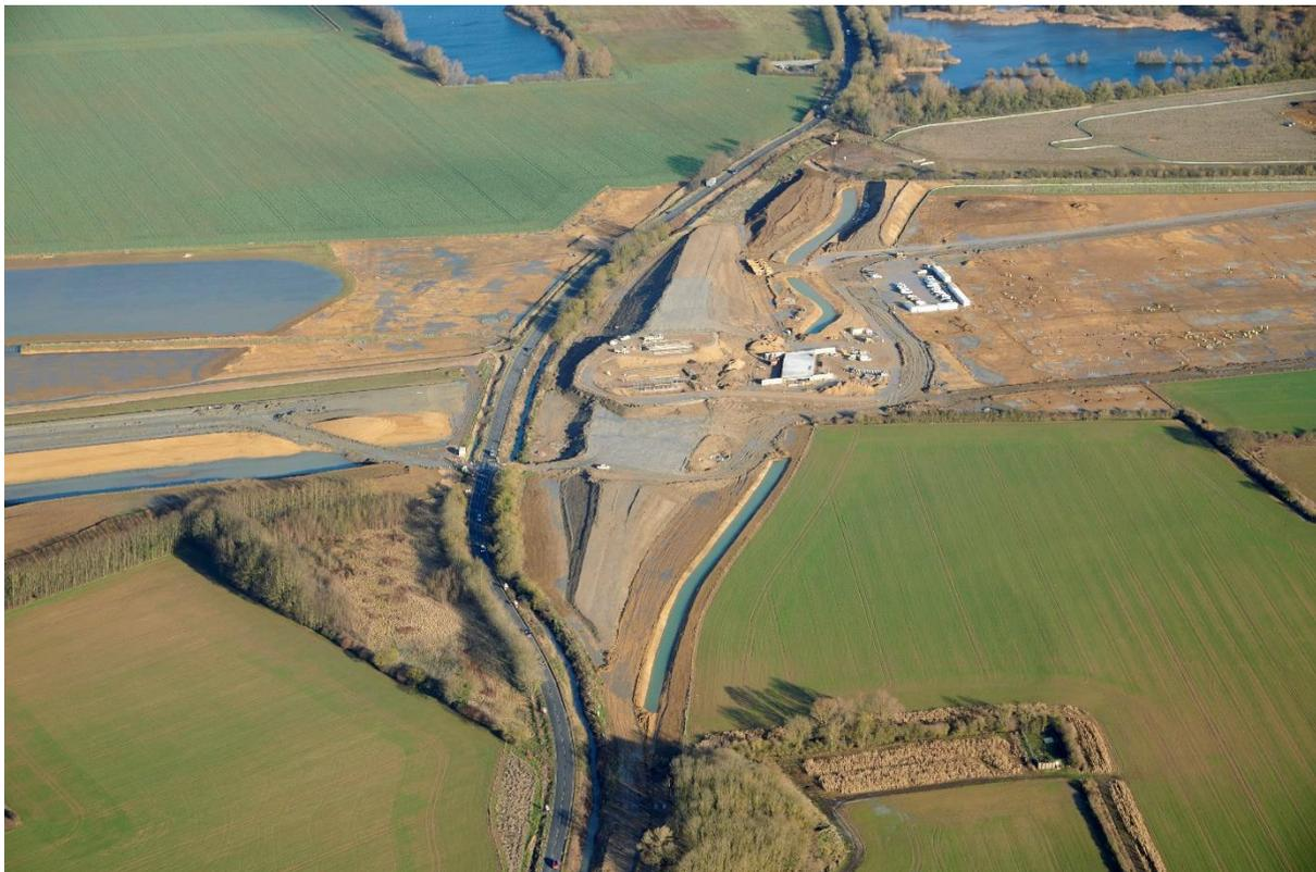
**Sections 4 & 5:** Work is underway to remove the temporary abutments which supported the bailey bridge at Swavesey junction. Construction of the permanent abutments next to the westbound carriageway at this location has started. This is in preparation for the installation of the first beams of the new bridge which will be built to the west of the current overbridge.
